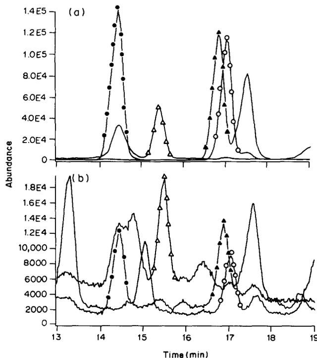
Fig. 1. SIM of TMS ethers of (a) authentic steroids: 5 $\alpha$ -androst-16-en-3 $\alpha$ -ol (●), and -3 $\beta$ -ol (○) at *m/z* 346 ([M]<sup>+</sup>), 5,16-androstadien-3 $\beta$ -ol (▲) at *m/z* 344 ([M]<sup>+</sup>) and 5 $\beta$ -androstan-3 $\beta$ -ol (△) at *m/z* 258 ([M-90]<sup>+</sup>), internal standard; and (b) Steroids in extracts from semen pool B. The ketonic functions were underivatized.
