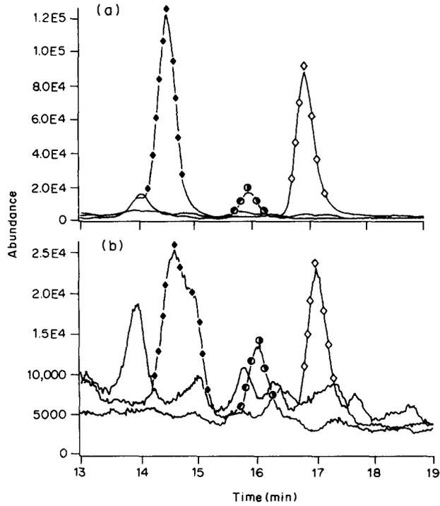
Fig. 2. SIM of (a) underivatized authentic steroids:  $5\alpha$ -androst-16-en-3-one ( $\blacklozenge$ ) at  $m/z$  272 ( $[M]^+$ ), 4,16-androstandien-3-one ( $\blacklozenge$ ) at  $m/z$  270 ( $[M]^+$ ) and  $5\alpha$ -androstan-3-one ( $\bullet$ ) at  $m/z$  274 ( $[M]^+$ ), internal standard; and (b) steroids in extracts from semen pool B.
